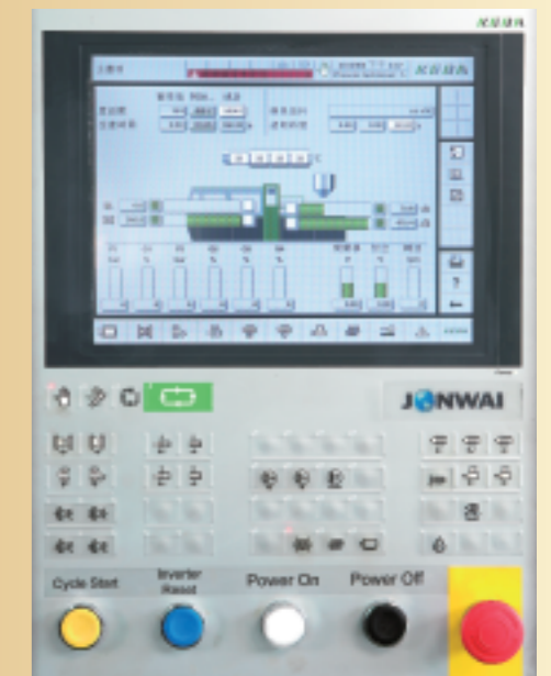
User Friendly KEBA Control Window based operation panel clear overview monitoring page. Modularized PLC design with widely function expandability.
